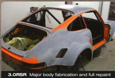
3.0RSR Major body fabrication and full repaint
